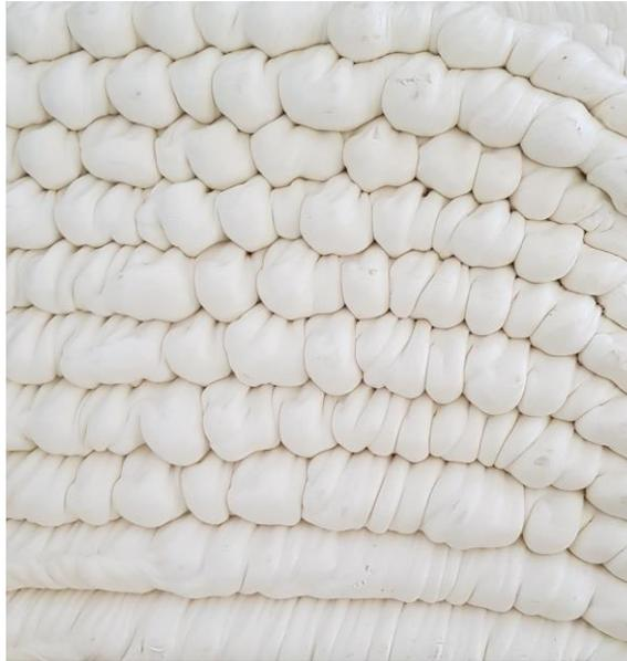
*Approx a meter height of a portion of a wall sample printed in polyurethane.*
