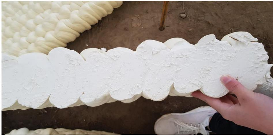
*Image of a section through the extruded polyurethane foam, showing the variation between different layers.*
